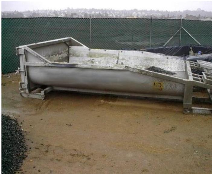
An example of a prefabricated concrete washout container
